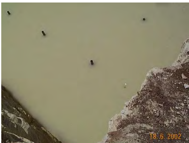
Figure 62: Vortex development in MDH soakaway under test (in line with boreholes)
