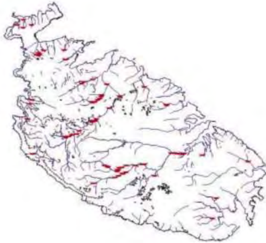
Figure 7: Map showing location and orientation of major valleys in mainland Malta (the marks in red denote the location of dams spanning across the valleys for water attenuation, retention, and recharge)
